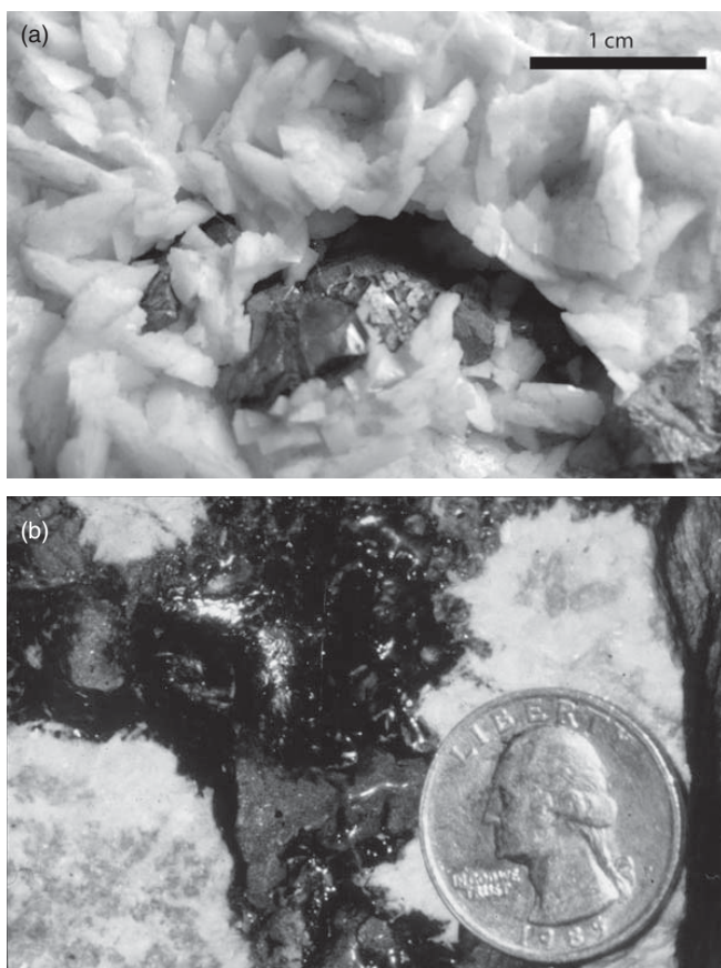
Figure 2.2 (a) The dark crystals of galena grew on top of smaller crystals of white dolomite. Whereas the dolomite contains almost no zinc, sphalerite contains as much as 64% by weight and is our principal ore mineral for zinc. (b) The dark material is solidified crude oil known as bitumen , which is lining a cavity in the white limestone. See color plate section.
